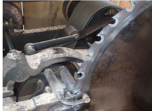
For those who are wondering . . . a Babbitt bearing is made up of a mixture of lead, tin, and antimonium. It creates a soft wear surface between the shaft and the heavy cast of the outer shell. Under optimal conditions, the clearance between the shaft and the bearing should be around 5,000 to 6,000ths of an inch, but with the wear, ours had grown to approximately 40,000ths of an inch.
