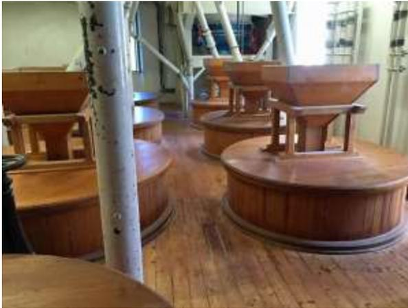
Plans are being developed to ship the millstones from Quebec to France next summer where they will be returned to working order by craftsmen whose principal work is dressing millstones, and where the metal bits which separate the stones from each other and connect to the drive mechanism will be improved to modern standards.
