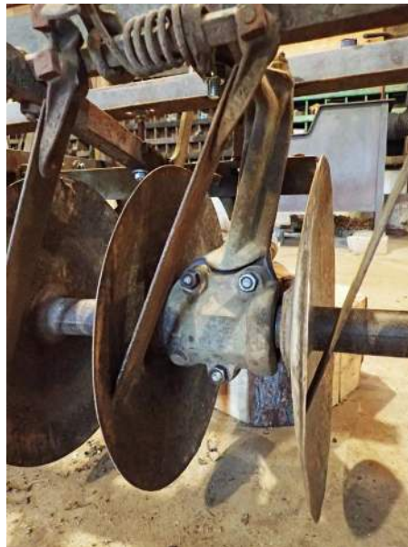
The new bearing sits inside the housing that holds the shaft of the disc harrow.
