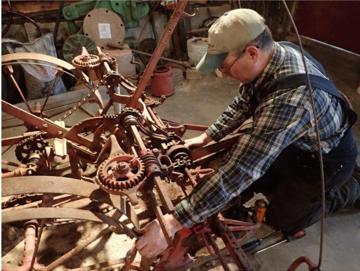
*Ray working on the gearing for the corn planter.*
