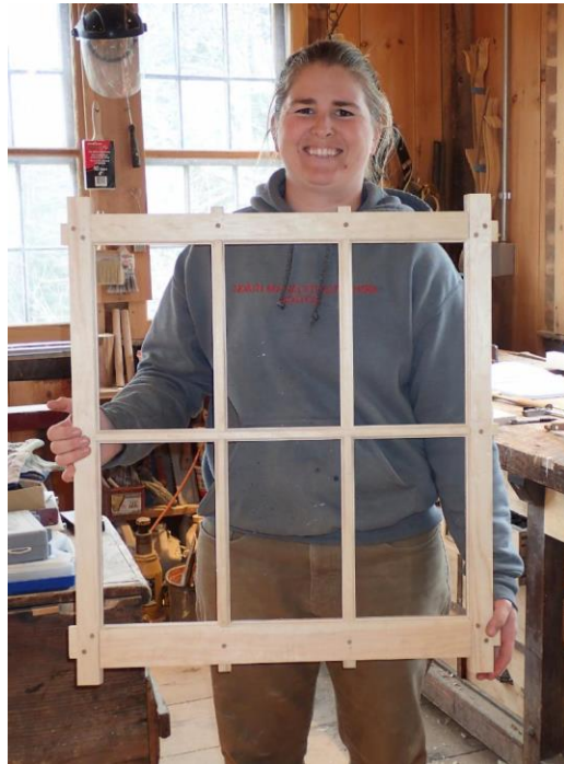
Emma with an assembled frame. The extra length on the stiles (called "horns") will be trimmed off before setting the sash in the window frame.
