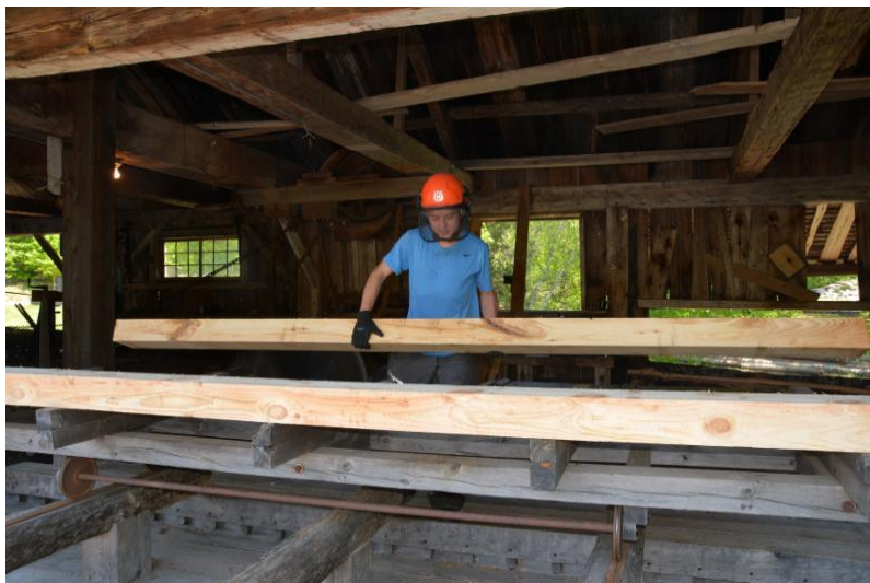
Millwright assistant Logan Clough stacking up newly sawed timbers that will be used for purlins or floor joints.
