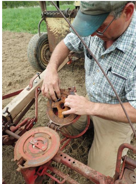
All old equipment needs frequent adjusting. Here Ray is checking the disc that governs the rate of corn kernel drop.
