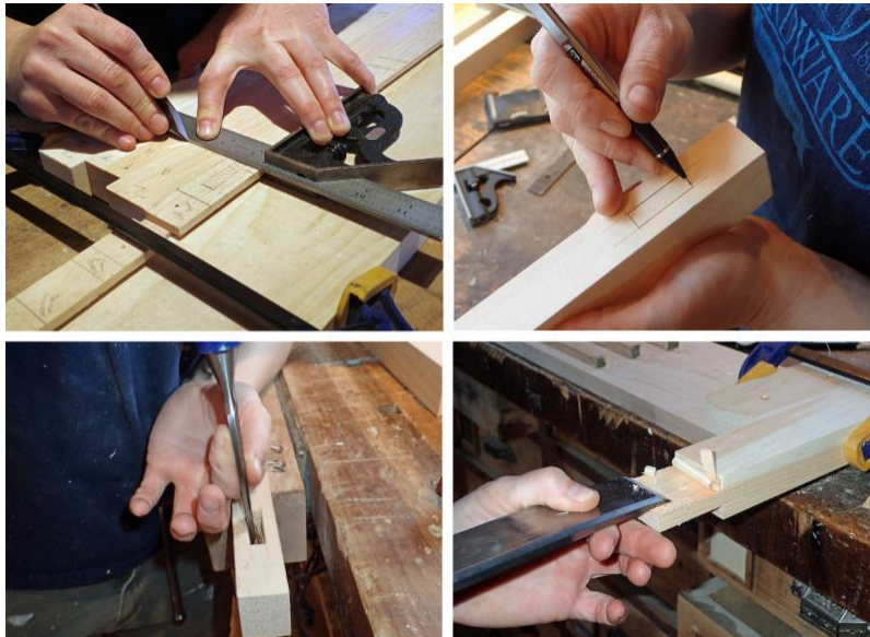
Clockwise from upper left: scribing the location for mortises & tenons using the story stick; outlining the mortise; cutting the mortise; and cutting the tenon.
