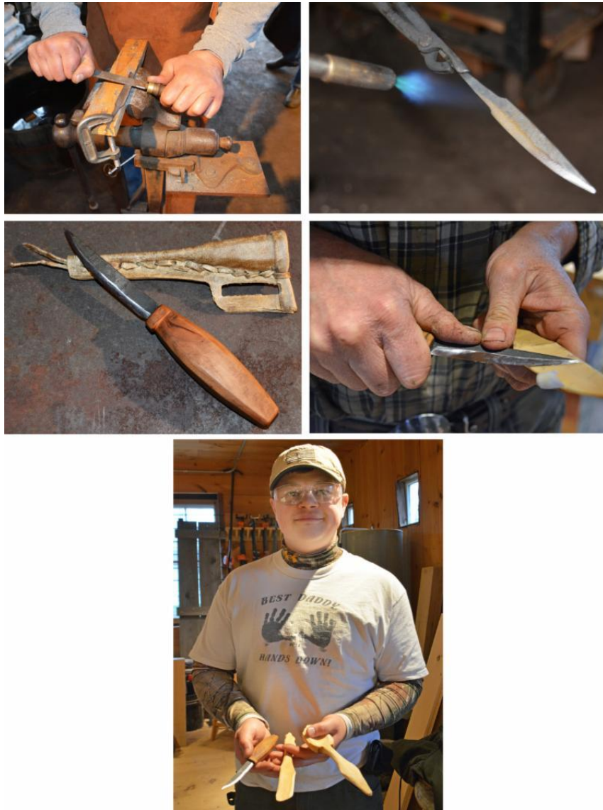
Left to right, top to bottom: Hand filing the bevel; heat tempering the blade; finished carving knife with sheath; whittling a butter knife; and Matthew Herrick of Henniker, NH with his completed carving knife, wooden butter knife and spoon.
