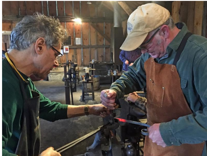
The Blacksmith Teaching Studio was busy with Garry Kalajian teaching students basic forging techniques and how to manage a traditional coal-fired forge.
