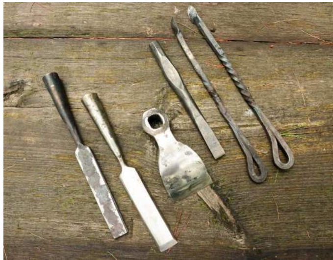
Joel Tripp taught a workshop in woodworking tools that challenged students to make a chisel and an adze. Some students made a punch and flux spoons as well.
