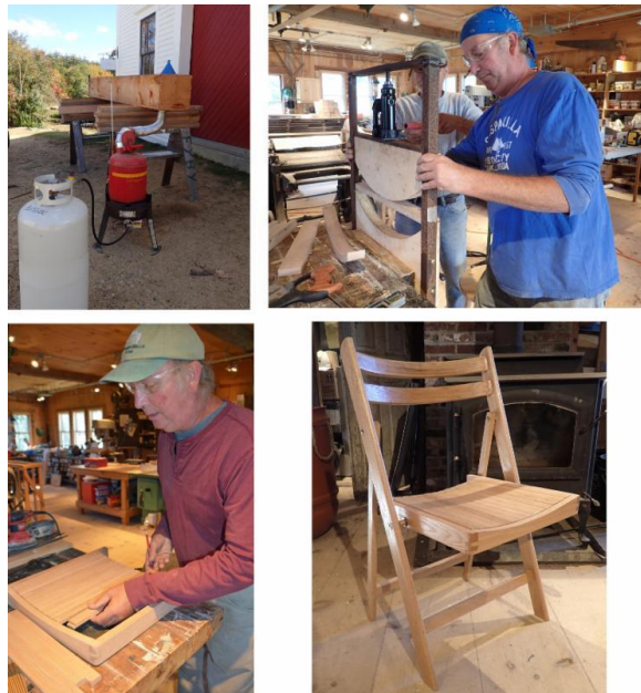
(clockwise left to right) home built steamer, Kevin Schurman getting ready to bend a piece in the jig, laying out the seat, a finished chair.
