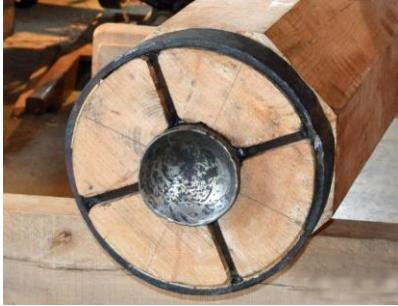
*Detail of the metal cap at the base of the shaft. (Photo BG)*
