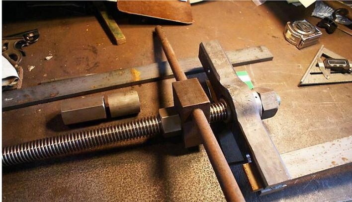
*Spreader with handle nut assembly. (Photo RS)*
