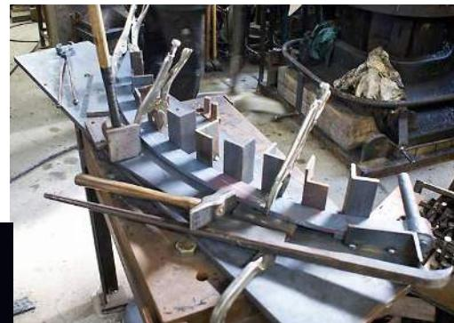
*Individual units welded to the jig creates the curve for the tongs. (Photo RS)*
