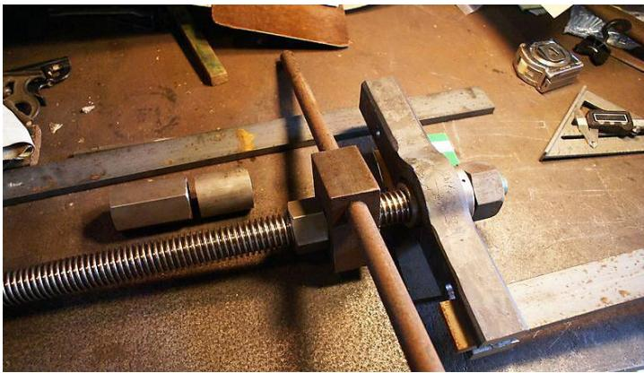
*Spreader with handle nut assembly. (Photo RS)*
