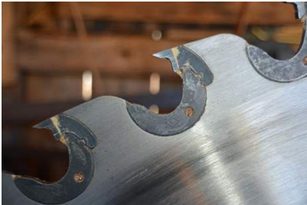
Close up of the new blade showing the shoulders & inset teeth.
