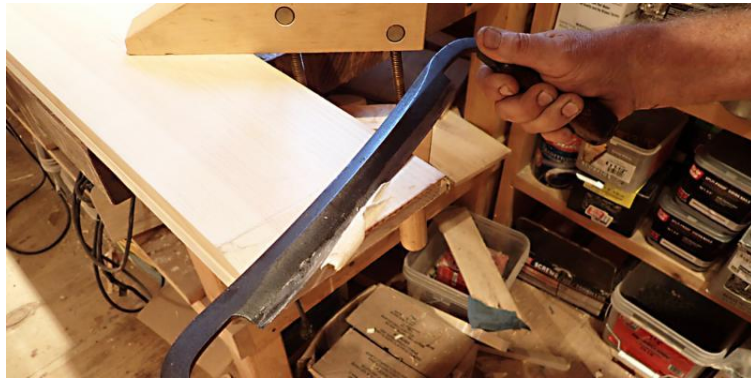
Skiving a clapboard with a drawknife.
