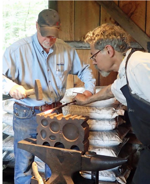
Garry Kalajian (right) & Jim Allen shaping a forge welded piece on a swage block.
